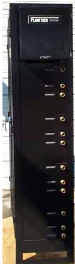
3/4" NPT outlet connections grouped by torch
